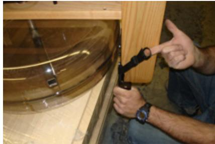
Secure the handle by looping an elastic band around one side, thread it under the top deck, and back over the other side of the handle.
