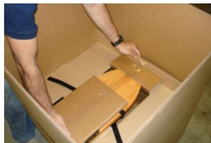
Step 3.) Pack the tank assembly. Secure the recoil belt by looping it around the forward riser bracket.
