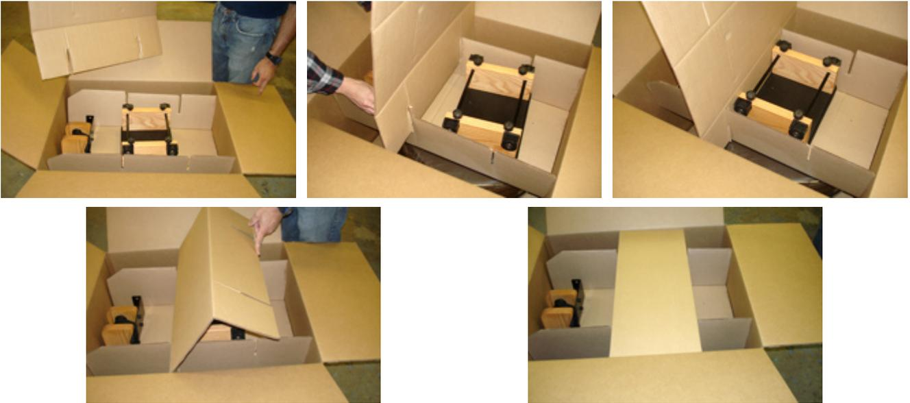
Step 6.) Place the siphon pump down the side of the box next to the tank and place the rear spacer, heel rests and bits bag in the cubby holes of the cardboard inserts.
